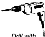
Drill with 3/16 inch Drill Bit
